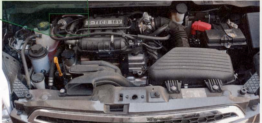
The 1.0 litre developing 68 hp makes a little room for LPG devices under the bonnet, such as the gas adapter and filter.
